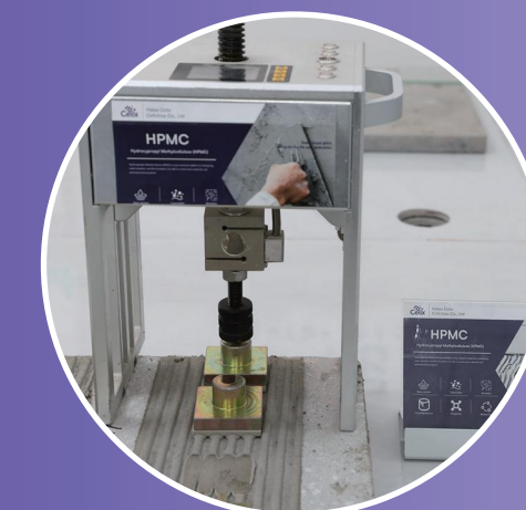
Tile Adhesive Pull-off Tester
